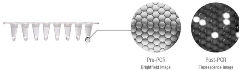
Step 2. Run PCR to endpoint. Quantification no longer relies on PCR kinetics
