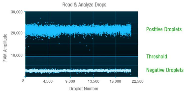
Step 3. Fluorescent analysis drop by drop (yes or no). Copy number calculated by Poisson distribution
