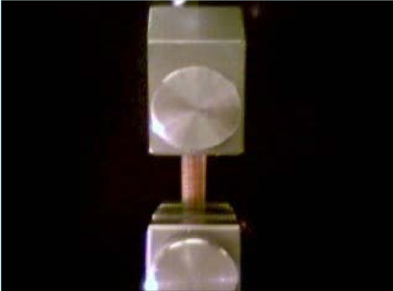
15 x 5 x 0.7 mm    500mm/min    100% strain    5 cycles
